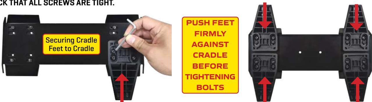
**STEP SEVEN** Turn the Cradle over onto the Cradle Feet. Place Cradles where you intend to use them before placing MX Dumbbell Handset into the Cradles.
